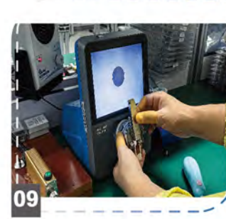
09 Check and clean module optical end face
